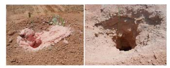
Figure 2 (L-R) Heavy ANFO after loading vs. ΔE after loading
